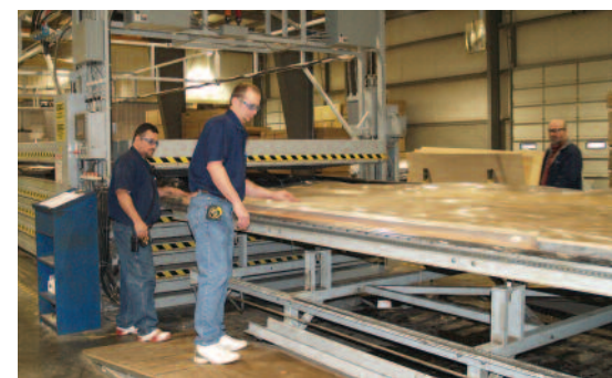
Dutchmen employees prepare a floor for vacuum bonding in the laminator. Shown from left to right are employees Jimmy Rivera and Dave Radcliff with Lamination Plant Manager Hank Johnson.
